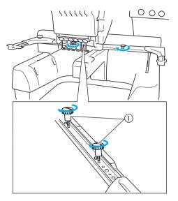
① Use the thumb screws removed in step ①.
